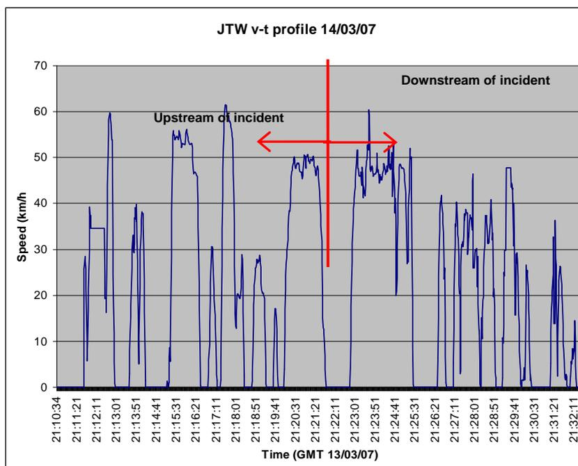
Figure 3 Probe vehicle speed time profile Glen Osmond Rd route, 14/03/07 'normal' day
