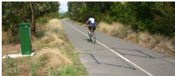
Figure 1: Automatic counter installation on a bike path (Source: VicRoads)
