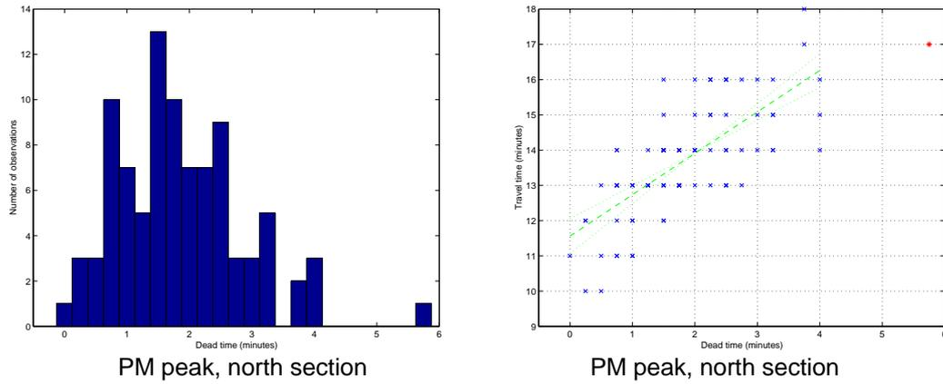
Figure 1: Diagrammatic representation of travel time and dead time. (Left) Frequency histograms of dead time. (Right) scatter plots of travel time versus dead time.
