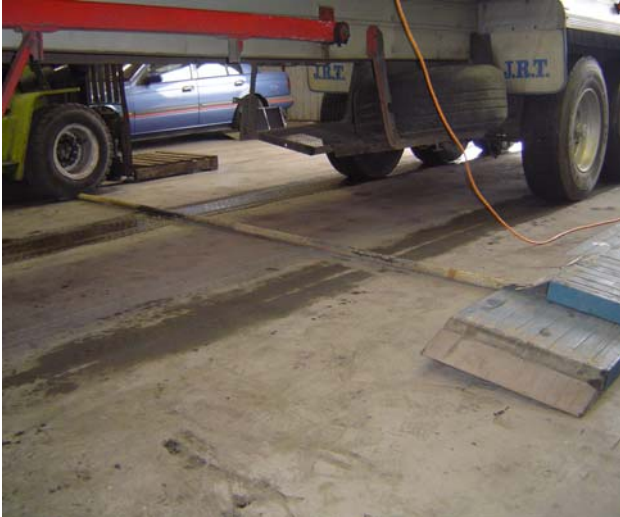
Figure 1 Pipe used for suspension vertical disturbance input.
