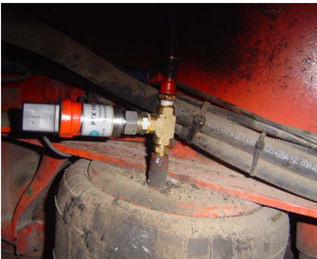
Figure 2 Pressure transducer location and plumbing details.
