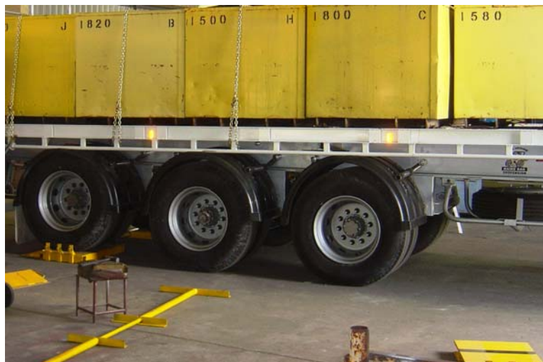
Figure 6 Showing the test masses on the semi-trailer with the pipe for the “pipe test” in the foreground, bottom left.
