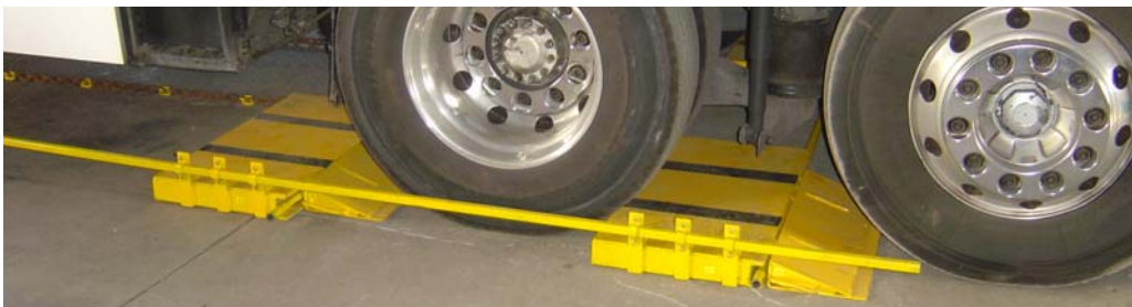
Figure 3 Before: showing preparation for the step test on the coach.
