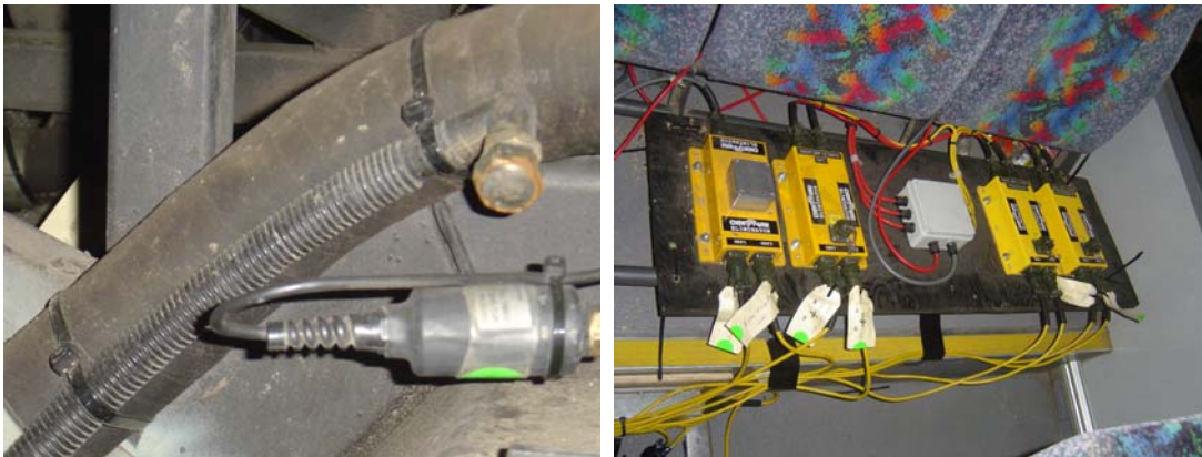
Figure 1 LHS panel: Air pressure transducers (green sticker) connected to air springs. RHS panel: CHEK-WAY® data recorders (yellow) used during the testing.
