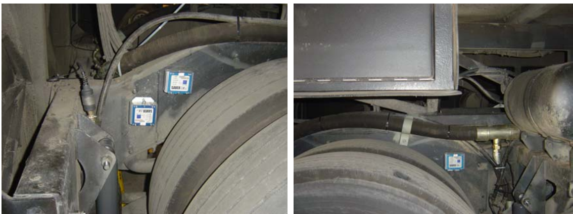
Figure 2 Lansmont SAVER™ 3X90 accelerometer/data recorders (blue and white) used during the testing.
