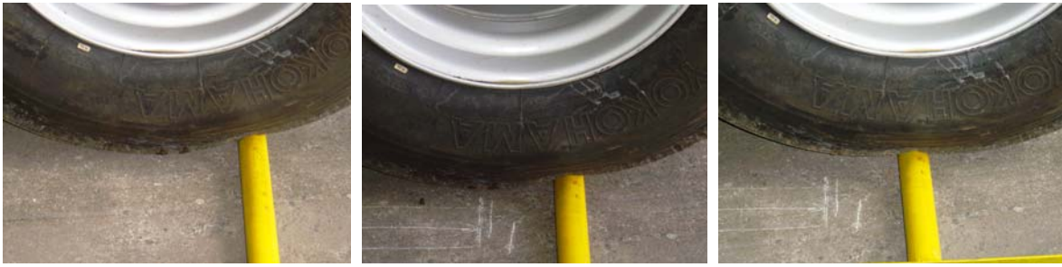
Figure 7 Detail of a typical tyre rolling over the pipe during the pipe test.
