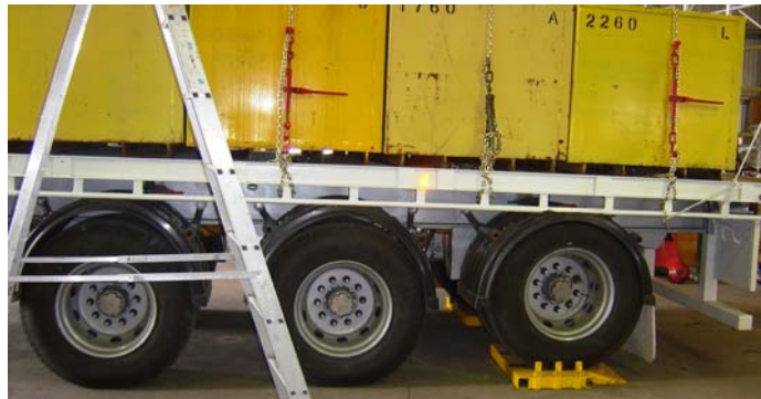
Figure 8 Showing the preparation for step-testing the semi-trailer rear axle only.
