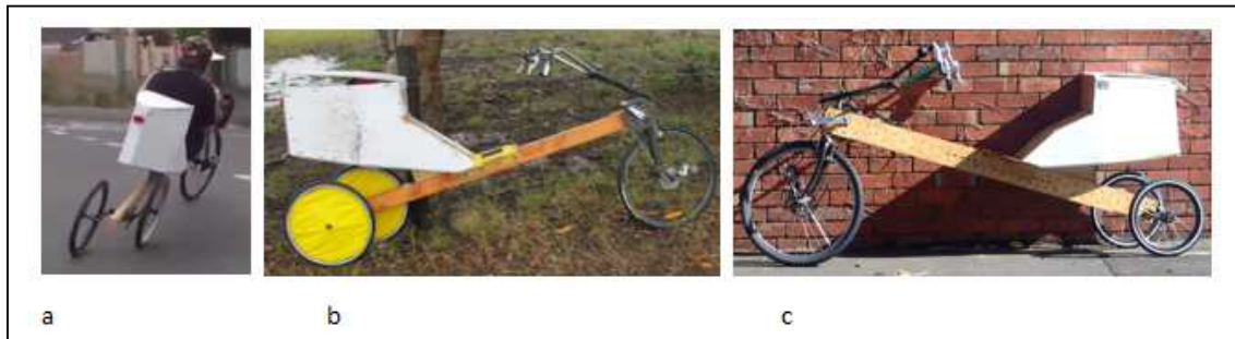
Figure 7: “Nurse leaning trikes, or NLTs: a, b) Solid timber frame & tailbox for luggage NLT1 c) Hollow plywood & tailbox NLT5.
