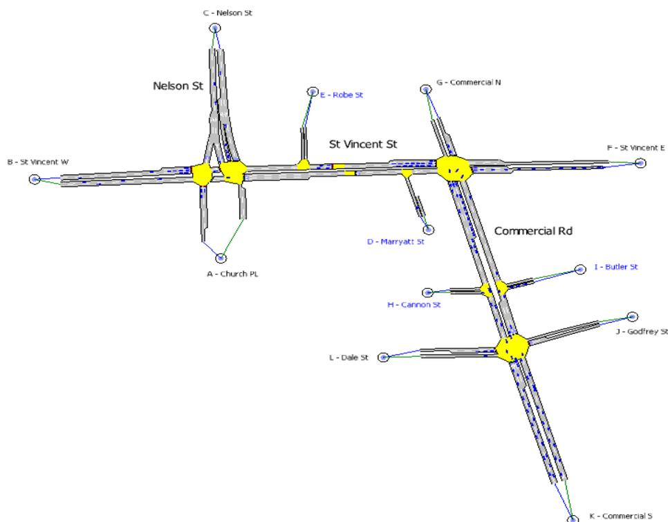
Virtually, the AIMSUN model is a stochastic representation of the base case LINSIG model, from which detailed traffic queue and travel delay information can be extracted. Importantly, the detailed vehicle behaviour and corridor traffic performance can be visualised and verified in a more user friendly manner.
