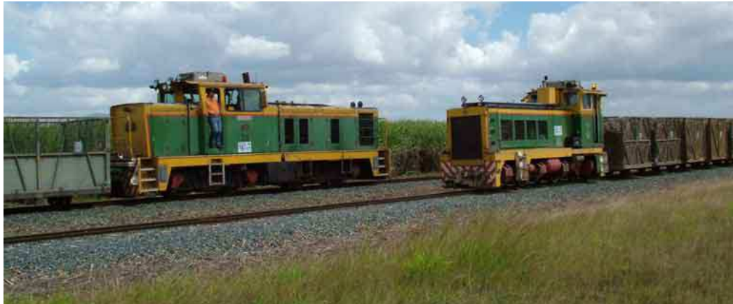
Figure 3 Various types of locomotives carrying empty and full rail bins
