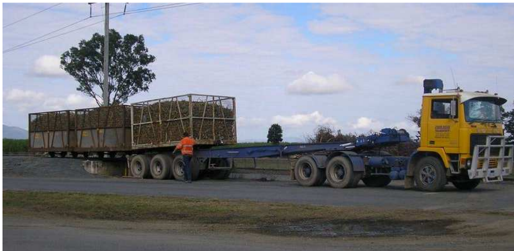
Figure 4 Tri-axle semi-trailer unloading bins at rail siding
