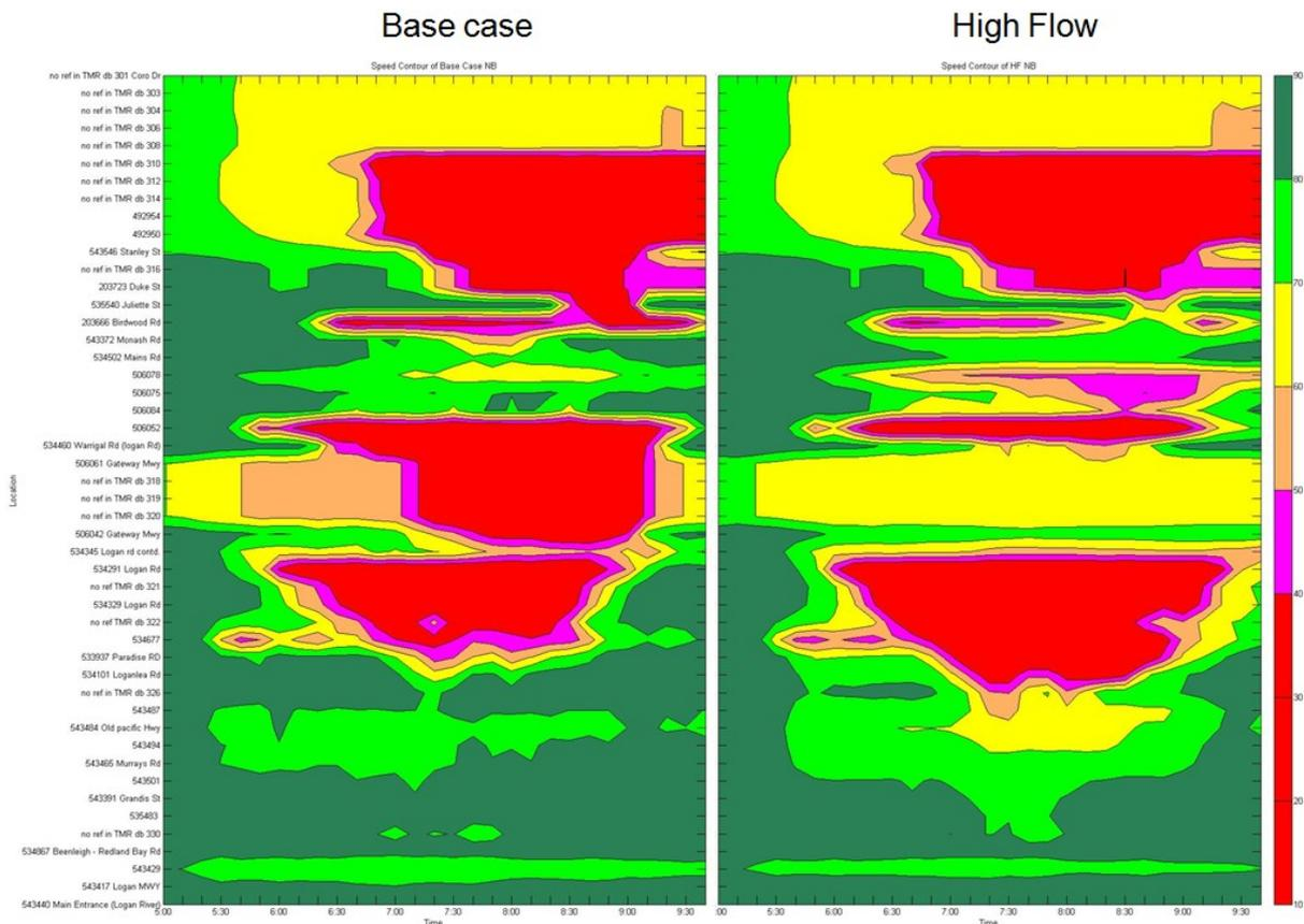
An analysis of Figure 8 indicates that most of the network experiences a slightly increased speed. However, the traffic situation from Murrays Road to Logan Road (12 sections in total) deteriorates (longer and expanded congestion) when VSL is activated. In this area, there are 6 on-ramps with high demand and 4 off-ramps with large flows, so a large number of lane-changing and merging are necessary. When VSL is activated, lower speed limits increase
