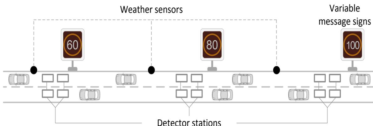
As shown in Figure 1, the components of a VSL system include:
