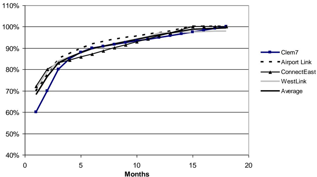
The actual and assumed ramp-up profiles shown in Figures 2 and 3 share a similar shape and define an envelope that characterises the “traditional” ramp-up profile of Australian toll roads during the era when toll charges when applied from Day 1. As shown in Figure 4, the key features of this “traditional” ramp-up profile are
