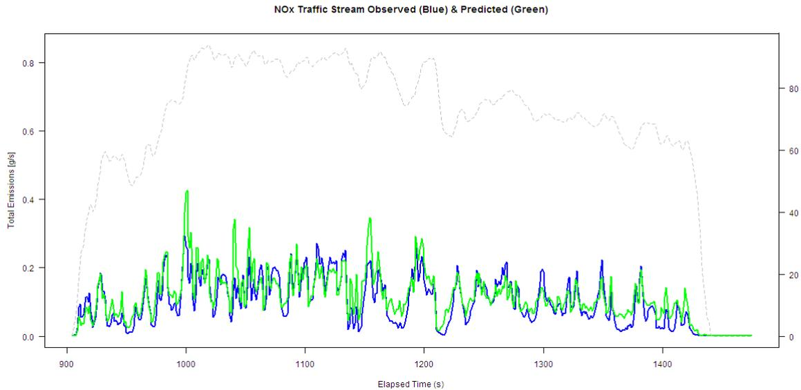
**Figure 5 – Time-series Plots for All 5 Vehicles Combined (1 Hz), Observed Total NO<sub>x</sub> Emissions (Blue), Predicted Total NO<sub>x</sub> Emissions (Green), Freeway Speed-Time Profile (Light-Grey Dotted Line)**
