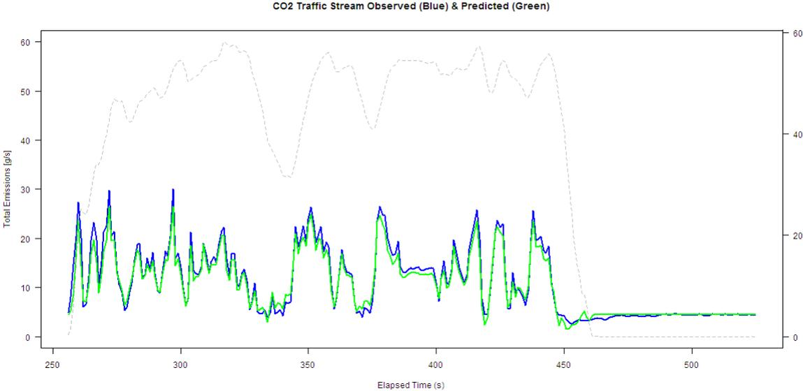
**Figure 4 – Time-series Plots for All 5 Vehicles Combined (1 Hz), Observed Total  $\text{CO}_2$  Emissions (Blue), Predicted Total  $\text{CO}_2$  Emissions (Green), Arterial Speed-Time Profile (Light-Grey Dotted Line)**
