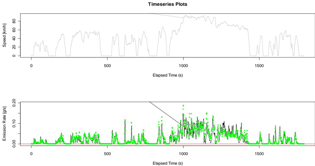
**Figure 2 – Time-series Plots for a 1988 Ford Falcon, Top Chart: Driving Cycle, Bottom Chart: Measured (Black Line) and Predicted (Green Dots) High Resolution NO<sub>x</sub> Emission Rates (1 Hz)**
