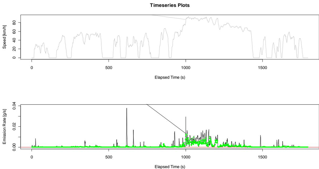
**Figure 3 – Time-series Plots for a 2001 Toyota Corolla, Top Chart: Driving Cycle, Bottom Chart: Measured (Black Line) and Predicted (Green Dots) High Resolution NO<sub>x</sub> Emission Rates (1 Hz)**
