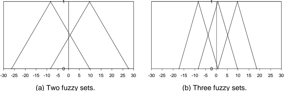
Figure 3: The membership function for the "Front Relative Speed" variable.
