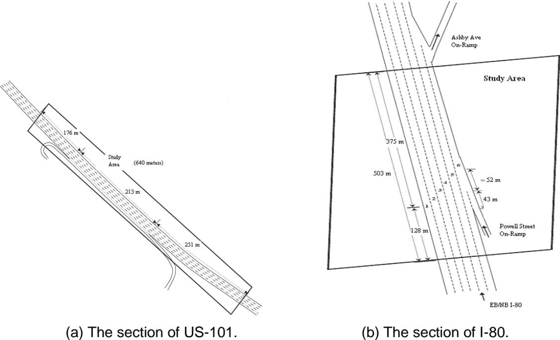
Figure 1: Schematic illustration of lane configuration for the two freeway sections.
