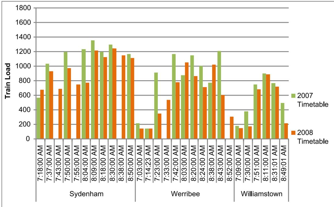
Figure 9: Comparison of train loads with two alternative timetables. The addition of more trains causes a reduction in loads, although these are mostly early in the peak.
