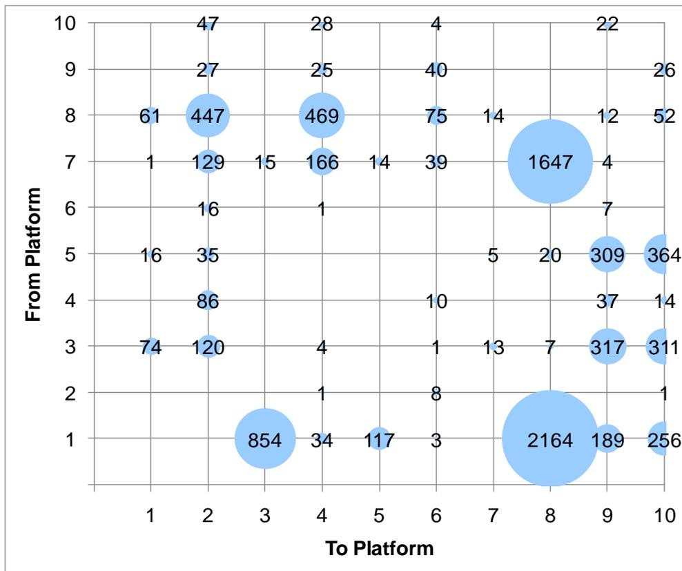
Figure 10: Volumes of transferring passengers between platforms at Richmond Station. The vertical axis represents the origin platform and the horizontal axis represents the destination platform. Platforms 7 and 8 represent a cross-platform interchange, whereas Platforms 1 to 6 do not. This type of diagram can be used to diagnose inefficient train presentation patterns at multi-platform stations.
