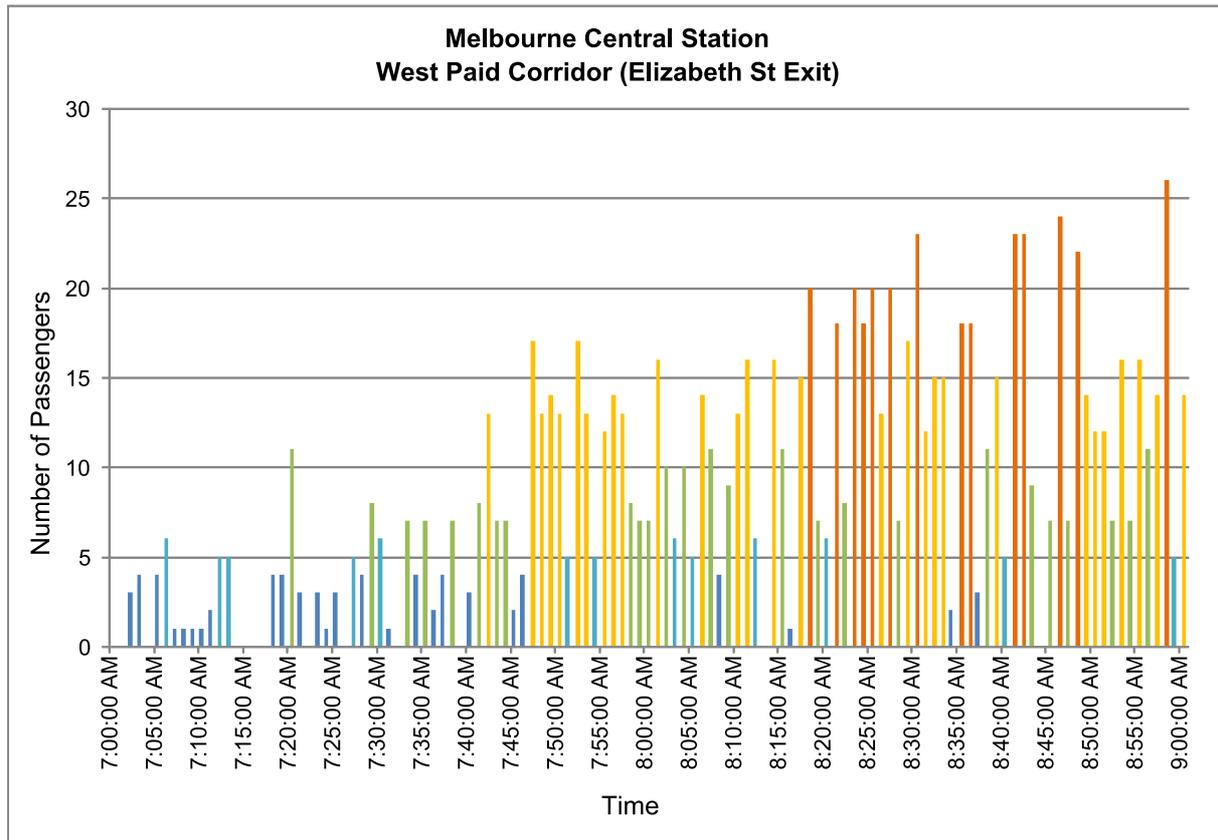
Figure 11: Pedestrian congestion plot showing instantaneous levels of service on a walkway at Melbourne Central Station. Walkway levels of service are defined in Fruin (1971).
