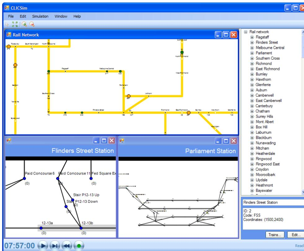
Figure 8: *ClicSim* user interface showing animation of trains (top pane) and internal station networks for two stations (lower panes).
