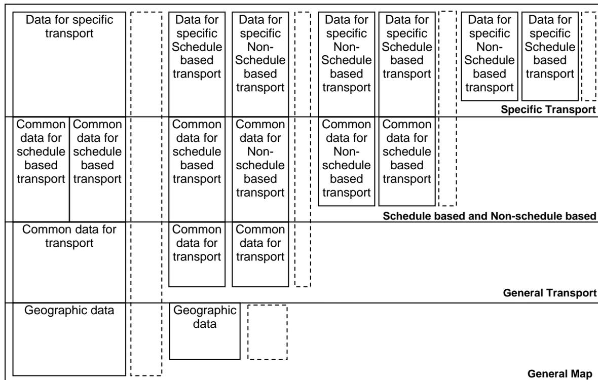
Figure 3: Physical structure of Four-layer database
