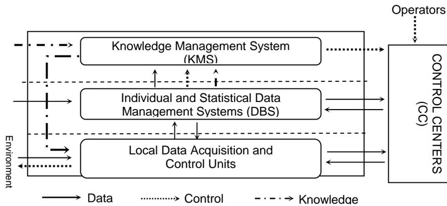
Figure 1: 3LOM architecture of Integrated Transportation System
