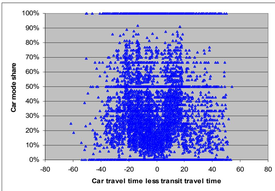
Figure 10 Car travel time less transit travel time versus car mode share
