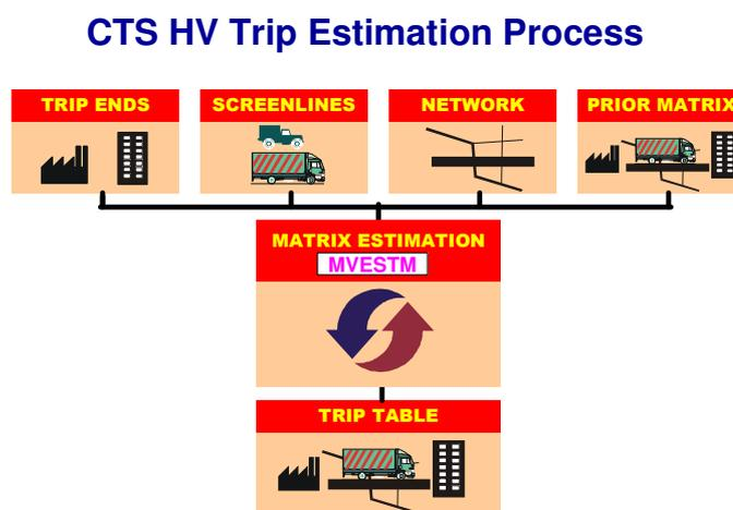
Figure 1 The CTS heavy vehicle trip estimation process
