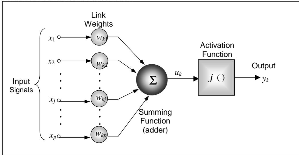
**Figure 1:** Non-linear model of a neuron
