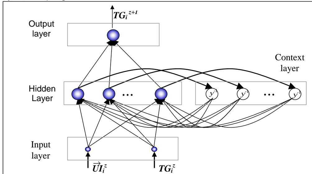
**Figure 5:** Application of an Elman NN for NGTM
