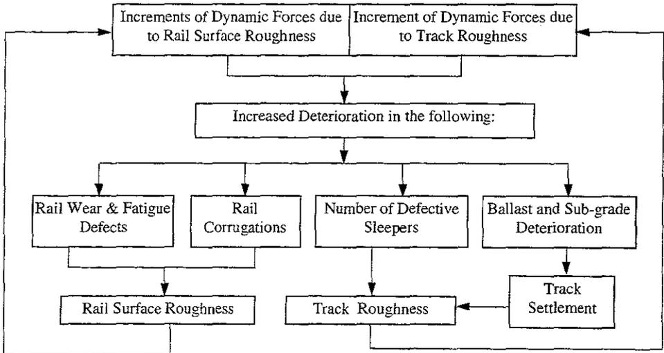
Figure 2 Interactions of deterioration of track components
