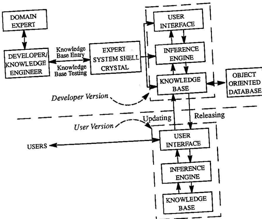
Figure 3. Two Version of the Expert System for Selecting Transport Planning Packages
