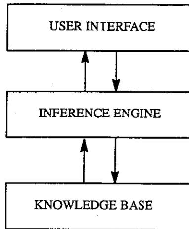
Figure 1. The Basic Components of Expert Systems
